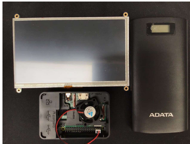
Figure 7. Power bank, Raspberry Pi and Touch Screen used as base station.
