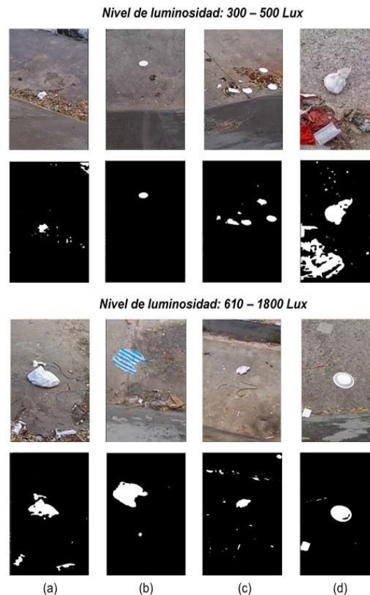
Figure 2. Waste detection through color segmentation. (a) Height of 1.5 m and inclination angle of 60°. (b) Height of 1.5 m and inclination angle of 20°. (c) Height of 0.5 m and inclination angle of 60°. (d) Height of 0.5 m and inclination angle of 20°.
